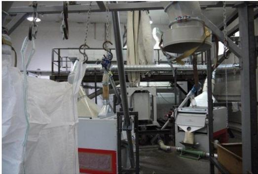
View of the unit's components, especially the screening and separating technique for cleaning the material from fabric remnants.
