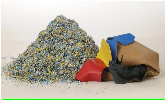
Industrial and previously used soft PVC recyclable materials, such as synthetic leather or swimming pool foils containing fabrics or textiles, are shredded, granulated and sifted, screened and separated. 100% of the resulting soft PVC recyclate is used in Caretta's fabric sheet and foil production.
