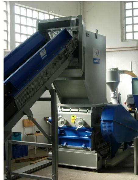
The shredded sections are then processed into granulate via a conveyor belt that is coupled to the volume intended for further processing. The screen used determines the grain size.
