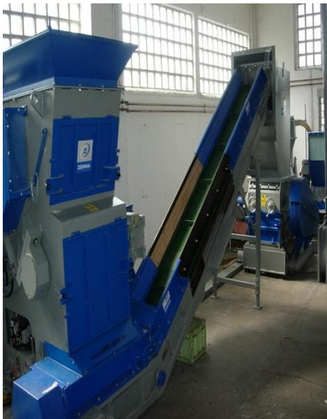
Recyclable materials clad with fleece, fabric or textiles are poured into a shredder from above and chopped into sections approximately 4 - 6 cm long. The system is geared to deliver 1,000 kg of output per hour.
